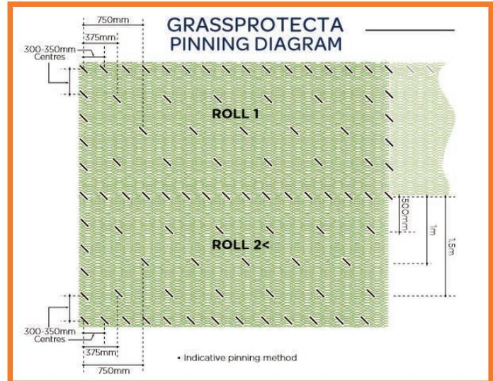
5. Position the mesh where required on the prepared surface. Starting from a corner of the roll and maintaining the mesh as taut and straight as possible at all times, fix the first edge (length) and then go back to the start and fix one end of the roll using the metal U-Pins (300 - 350mm centres). Do not fix both ends or both edges at this stage. Always work in the same direction along the mesh length to keep the mesh taut and to avoid ripples.
