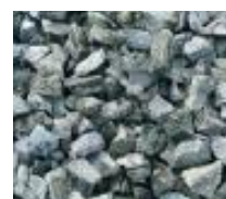
CGA Type 4/20 (clean stone) - permeable
